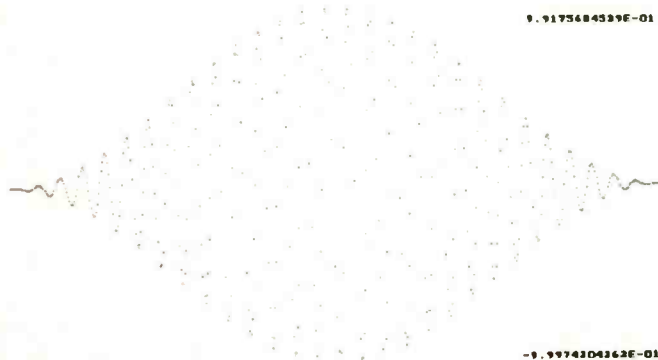
Fig.7. Using windowing to reduce the effect of discontinuities: a Hann window applied to an 1106Hz signal, seen in the time domain.
