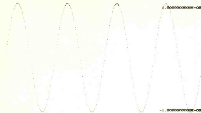
Fig.3. With this 150Hz signal, the blocks of sampled data represent a whole number of cycles.
