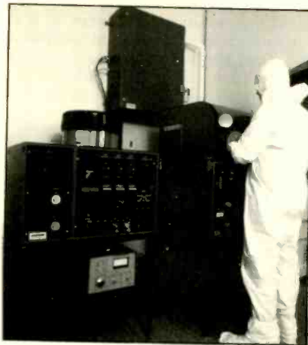
Unwanted metal is etched off the wafer by dry-etch plasma machine.
