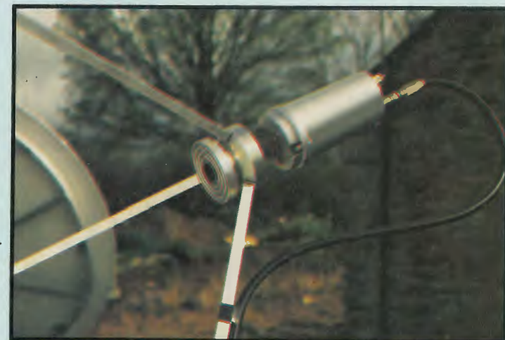
Polar mount rear support structure can be fitted with motor and remotely controlled from the tv set or simply hand operated with lead-screw to reduce cost.
