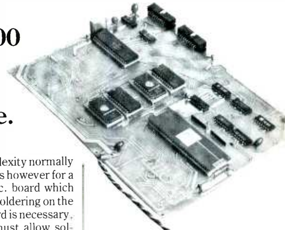
Our front cover shows the 68000 board in its fullest form with G64-bus interface — this is the basic version.
