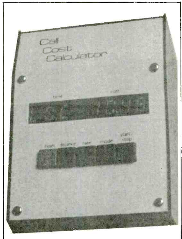
The calculator displays elapsed time and cost of calls in progress and stores running totals in memory.
