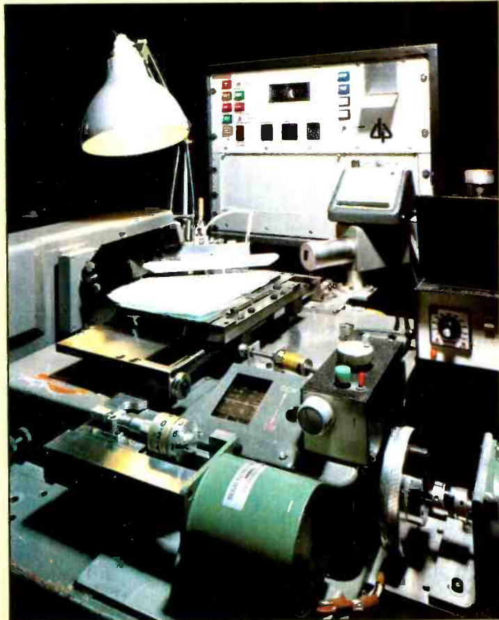
Setting accuracies of \pm 0.1 minutes of arc prior to cutting are needed in positioning quartz to achieve the required performance.
