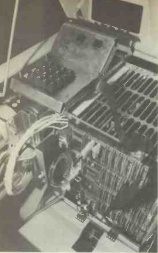
Engineer's console of microprocessor-based disc-drive showing keypad and display becomes accessible only with the cover raised.
