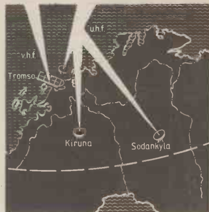
Fig. 2. Arrangement of radar systems in the EISCAT scheme. In the v.h.f. system the transmitter and receiver are in Tromso. The u.h.f. system, however, has a transmitter in Tromso and receivers at Tromso, Kiruna and Sodankyla. Both transmitters have a repertoire of pulse modulation waveforms to match the differing requirements for space, time and frequency resolution in various parts of the ionosphere.
