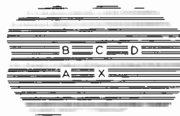
Fig. 6. Simple predictive codings can be improved in various ways. In predicting the X pel, elements can either be averaged, e.g. (A + D)/2 , or based on differences between lines, such as A + (C - B) .
