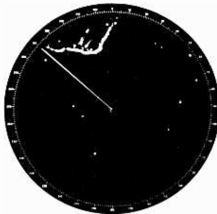
Photographs show the improvement obtained with Decca's new Clearscan radar circuitry. Above, the improved picture.
