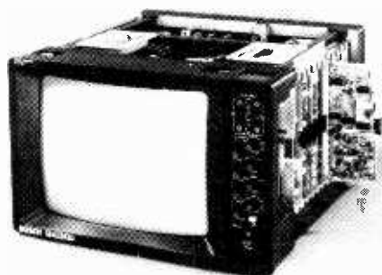
Fig. 1. The new colour monitor from Bosch Fernseh. The basic instrument can be expanded by the addition of plug-in boards into a PAL, NTSC, SECAM, or PAL-M monitor; in one form it may display the input test signals as levels.
