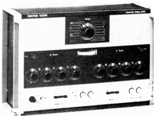
The B224 is a manually operated bridge, the resistive and reactive terms being independently set to a null indicated on the meter. A rechargeable battery is fitted in order to make the instrument portable.
