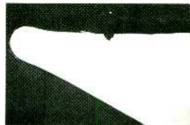
Sectioned iron-plated bit, after 40,000 simulated operations using SAVBIT Solder.
