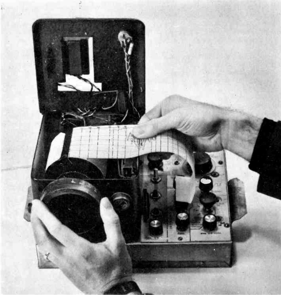
Showing how the chart is attached, by a folded tongue in the paper fitted into a slot in the drum.
