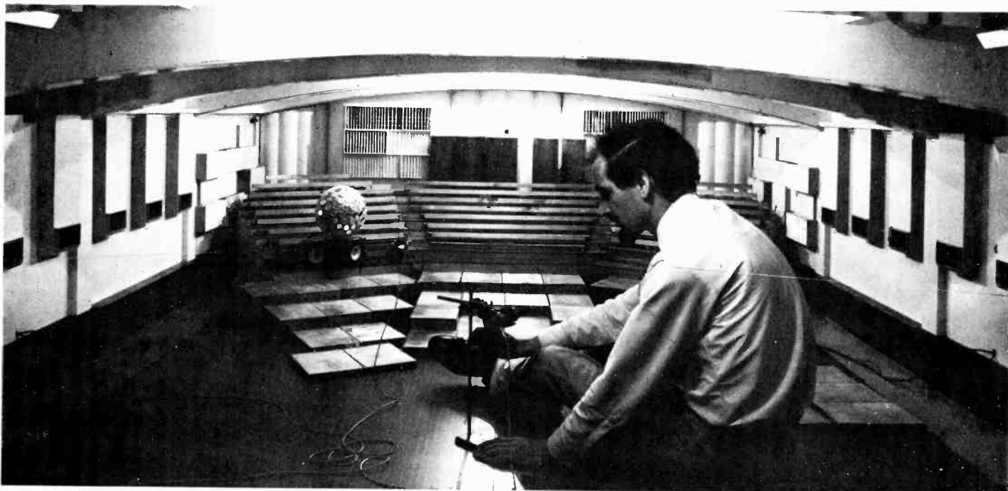
This 1/8-scale model of a studio has been used by the B.B.C. in listening tests to determine how the acoustics of the real studio might be improved.
