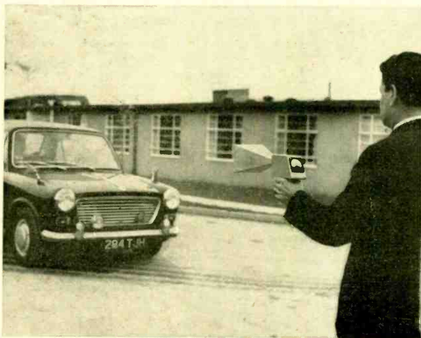
(below) Intruder alarm, showing warning lamp on top. The Doppler radar set inside uses a horn aerial giving a moderately wide beam, and has a range on a man of about 50 yards.
