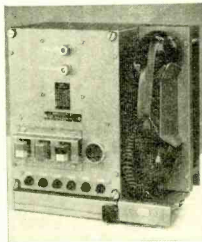
Drivers on the London Transport Victoria line and its Brixton extension will be able to communicate directly with other trains using a v.h.f. radio link. So far Nelson Tansley Ltd., 144 Holland Park Avenue, W.11, have received orders for about 170 communication systems as shown in the photograph. These, in addition to inter-train communications, offer passenger address and cab-to-cab intercom facilities.
