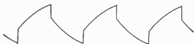
Fig. 6. Waveform of Fig. 2 (a) modified by use of poor quality electrolytic capacitor with high series resistance for C_1 .
