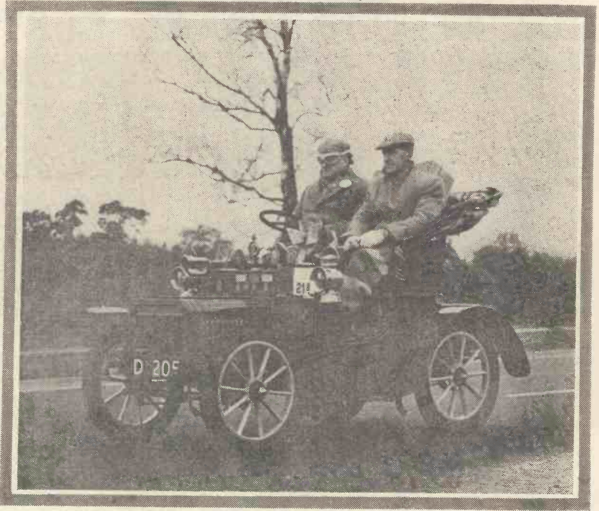
1904 Humberette Two seater. Single cylinder 6½ H.P. Beeston Model. Owned by P. Newington, Esq.
