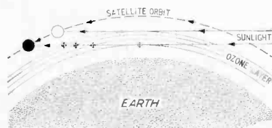
Fig. 3. Attenuation (recorded by ionization chambers) of sunlight through the atmosphere provides a measure of absorbing gas (oxygen).
