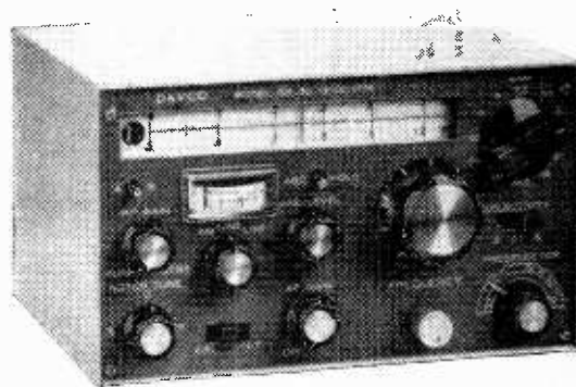
Above: Fig. 4. Compact communications receiver by Davco (U.S.A.) using field-effect transistors in the front end.
