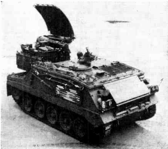
Green Archer mortar locating radar equipment identical to that already in use by the British and Swedish Armies is to be sold to the West German Government. Twenty-five sets of this equipment, worth about £3M, are to be supplied by EMI Electronics Ltd., of Hayes, Middx. Several other countries are evaluating this equipment, which pinpoints enemy mortar firing positions by plotting the bombs in flight. The illustration shows an installation fitted to an armoured fighting vehicle.
