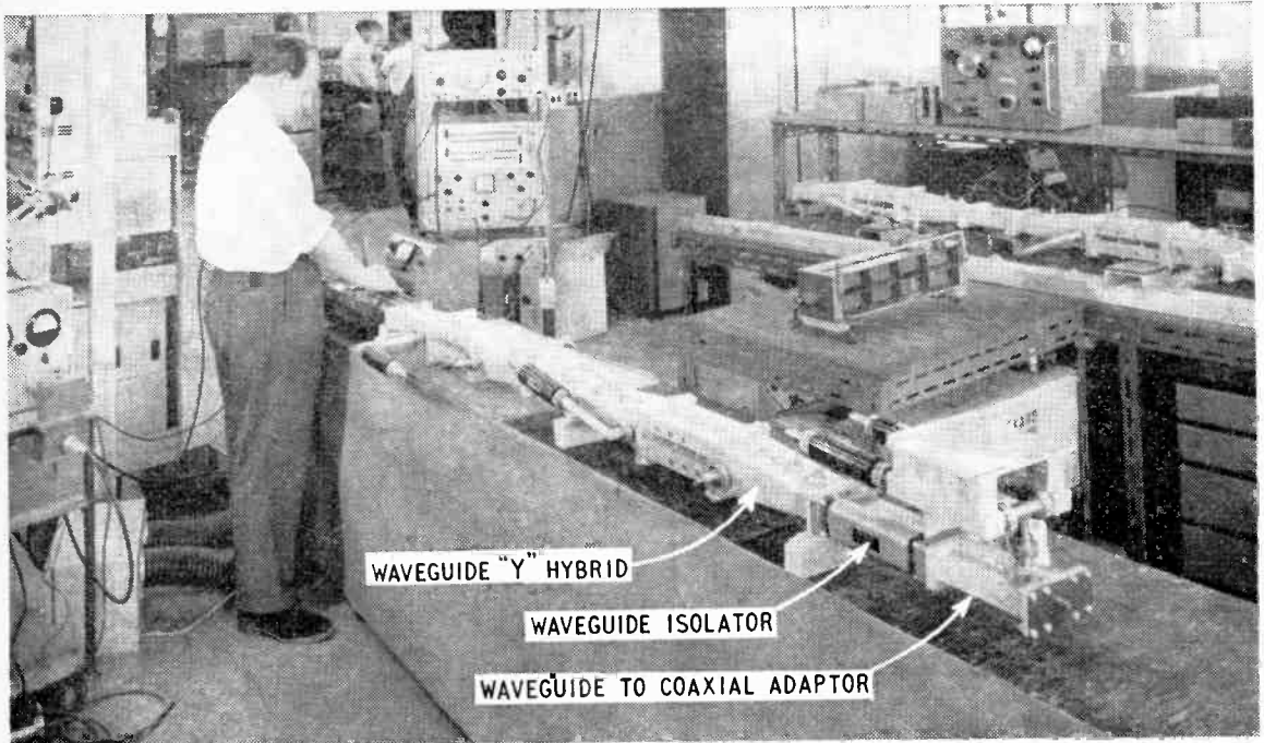
Aligning a 2,000 Mc/s radio link waveguide duplexer.
