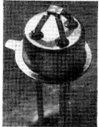
The S.T.C. BSY95 made by the new process.
