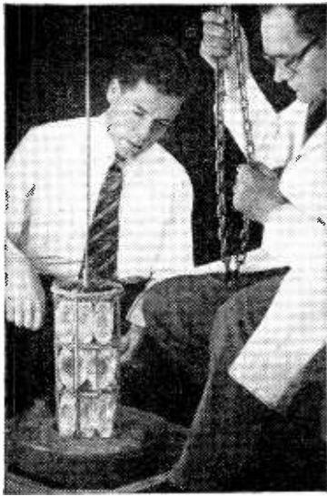
Using a high-pressure process, Standard Telephones and Cables are manufacturing synthetic crystals at their Harlow, Essex, factory. The process takes three weeks.
