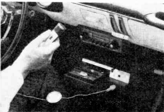
▲ Paper masks are provided for locating test points in Graetz printed circuit receivers (in this case the "Super Page").
