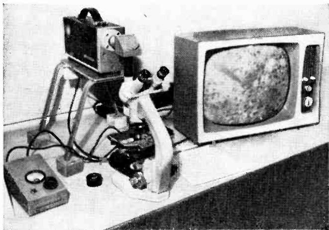
Watson television camera microscope eyepiece used with a trinocular microscope.
