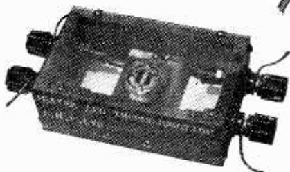
A.M.F. thermojunction ammeter in display box.
