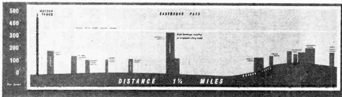
Typical radio path eastwards from the lowest aerial on the proposed tower which, as is shown, would just clear the highest proposed building in that direction.
