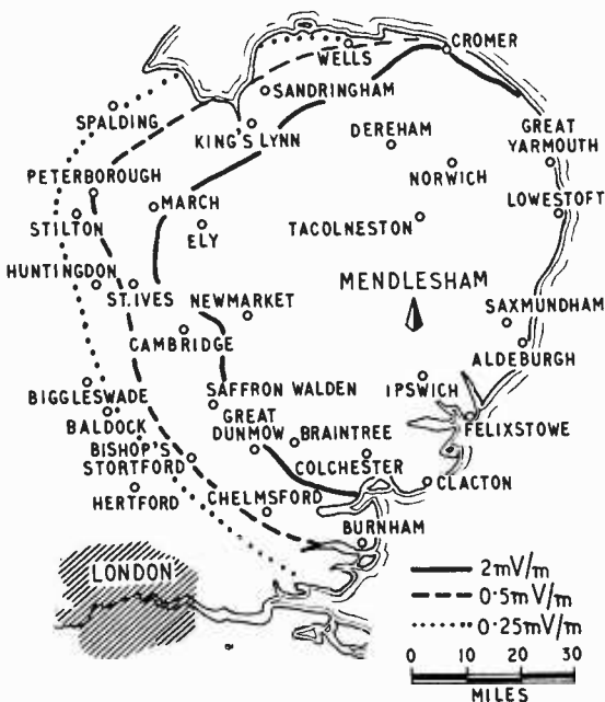
ESTIMATED COVERAGE of the I.T.A.'s East Anglian station being erected at Mendlesham, Suffolk. It will radiate in Channel 11 when opened toward the end of this year, the transmissions being horizontally polarized. Its maximum vision e.r.p. will be 200kW.
