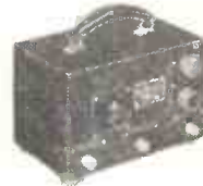
Range Calibrator BC-949; contains a resonating circuit that can be switched to produce signals from 8 to 81 kc/s. Valves: one each 6SL7GT and 6H6.
