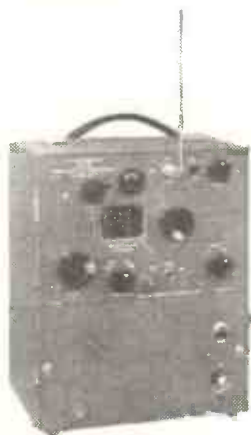
FM-3 Frequency Meter Portable direct reading meter measures 1 to 1,000 mc., generates 20 to 1,000 mc. Accuracy \pm 0.001\% . Also available with external power supply and rack-mounted.
