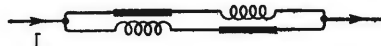
Fig. 8. Two cryotrons in transposed series connection, forming a bistable trigger circuit. For clearness the control coils are shown beside the "gate" wires instead of wound around them as they actually are.
