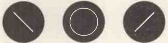
Fig. 2. Appearance of trace for phase difference increments of 90°. The centre circle corresponding to 90° or 270°.
