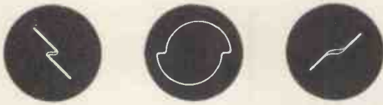
Fig. 3. When using the erase head without bias for recording, the waveform is distorted but still indicates phase.
