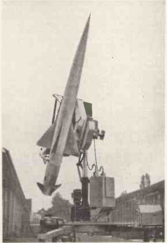
Fig. 4. A "beam-riding" missile on its launching ramp.
