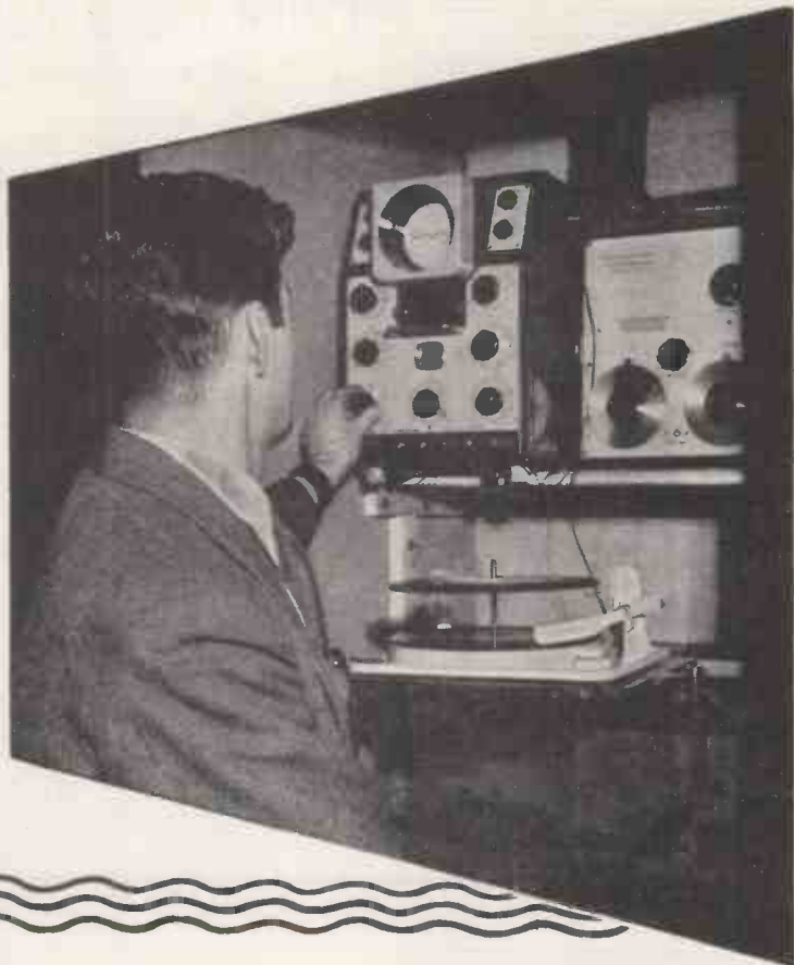
One of a line of testing booths where the final electronic test is carried out.
