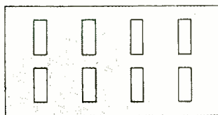
Left: Fig. 2. An array of slots in a screen complementary to Fig. 1.
