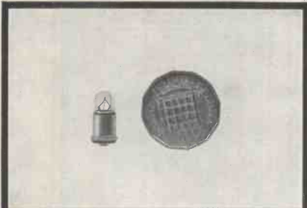
ATLAS MIDGET PANEL BULB Overall length: 14.6 mm. Bulb diameter: 6.3 mm. Rating: 28v., 1 watt, 0.04 amp. Also available in 12v., 6v. R.A.E. and S.R.D.E. type approval. Flanged cap and single centre contact for easy replacement.
