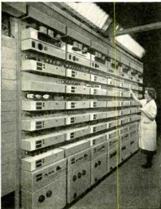
Fig. 1. Receiving valve life-test bays.
