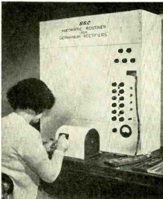
Fig. 8. Automatic routiner used for testing germanium diodes.
