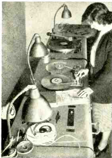
PLAYBACK console for tape and disc recordings at the Berlin Station RIAS (Radio in the American Sector) which radiates on a frequency of 989 kc/s with a power of 100 kW.
