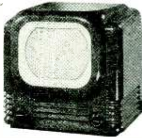
Baird portable television receiver, Model TI65, which utilizes the mains lead as an aerial.
