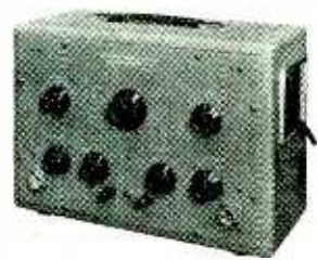
(Right) Avo universal bridge for measuring inductance, resistance and capacitance.
