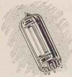
Bulb diameter \frac{3}{8} in. max. Seated height, 1\frac{1}{2} in. max.
