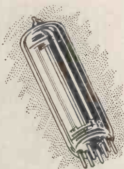
Bulb diameter, \frac{3}{8} in. max. Seated height, 2\frac{1}{2} in. max.
