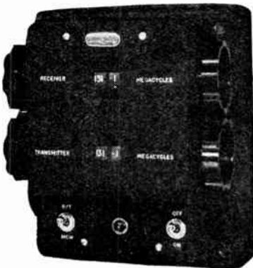
Control Unit of Murphy 140-channel v.h.f. transmitter-receiver. In each case one knob selects the whole number and another the decimal part of the operating frequency.
