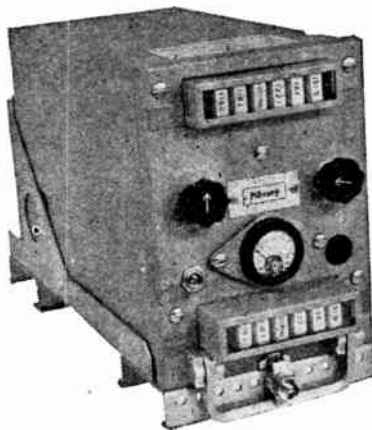
Plasley PTR61 lightweight aircraft v.h.f. equipment providing six crystal-controlled channels.
