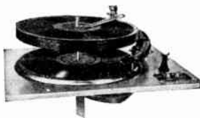
Collaro RC500 rim- drive automatic record-changer.
