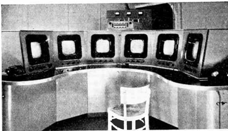
Display console with centralized operating controls.
