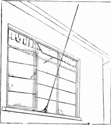
The illustration shows the "WINROD" aerial L.581. Price 19/6. It is neat, inexpensive and easy to fix. An outdoor aerial of this type will always improve signal-to-noise ratio in relation to indoor types.
