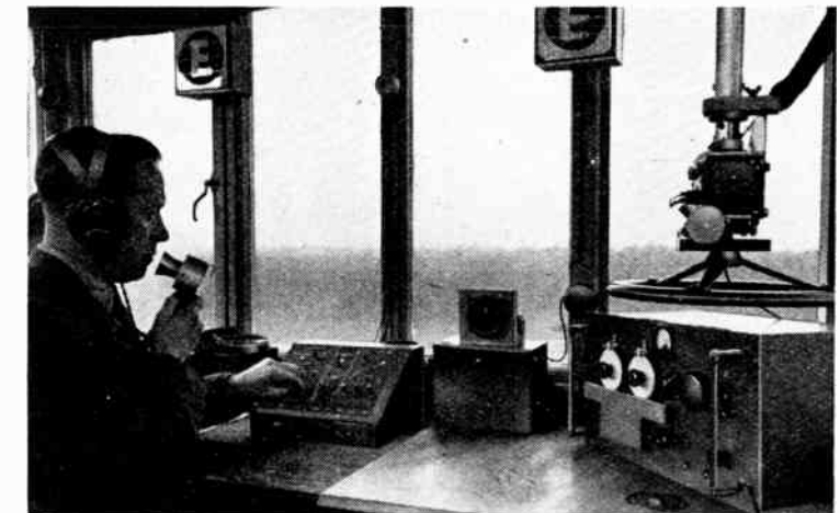
V.H.F. direction finder installed by E. K. Cole in the control tower at Southend airport. The aerial control wheel is visible on the right immediately above the D.F. receiver.
