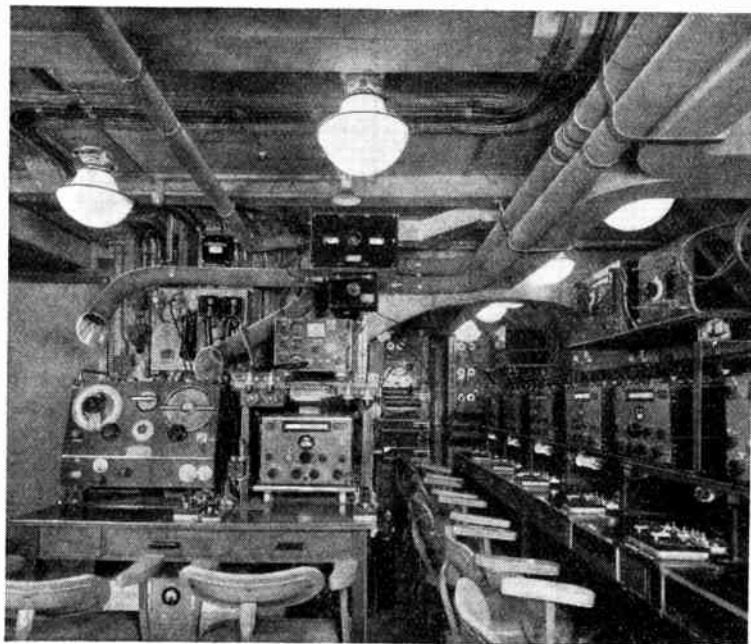
Bridge Receiving Room of an aircraft carrier. All-wave receivers are mounted in a row above the operators' bench on the right. The larger set in the left foreground is the medium-frequency D.F. outfit.
