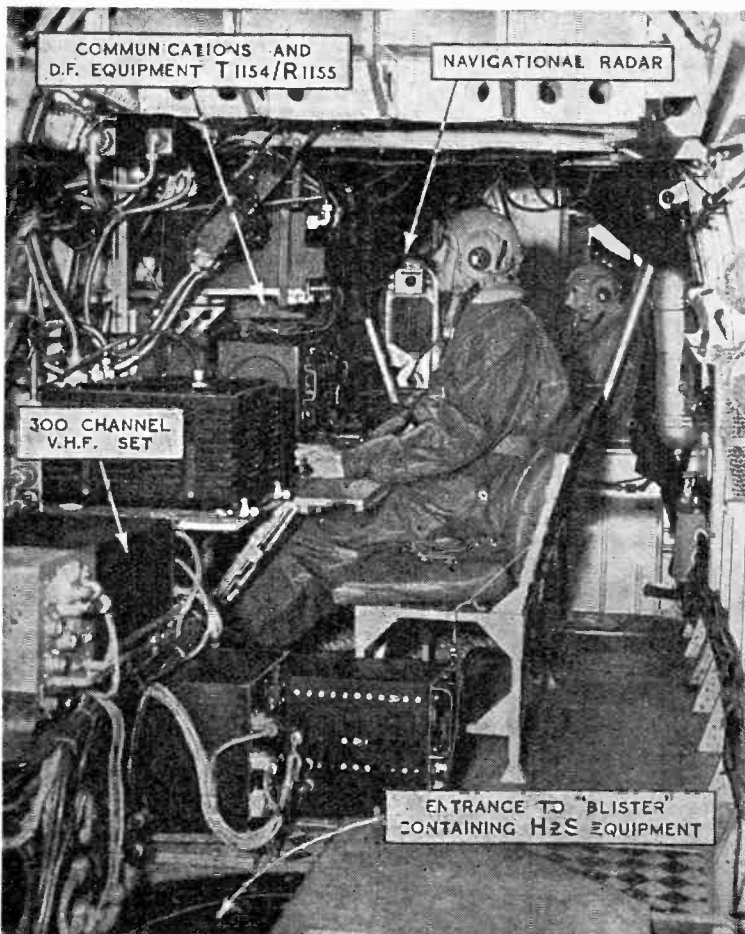
Interior of the converted Halifax bomber showing the location of the principal items of radio equipment.
