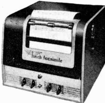
The Finch facsimile receiving unit which reproduces pages a little larger than those of Wireless World at the rate of thirty an hour.
