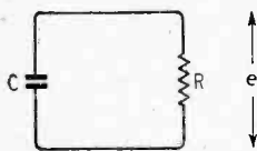
Fig. 1. The basis of a time-base. A charged capacitor is allowed to discharge slowly through a resistor.
