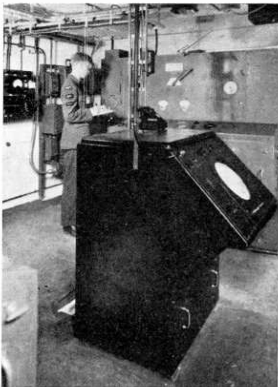
Underground radar stations combined the dual functions of locating enemy raiders and the control of our fighter aircraft.
