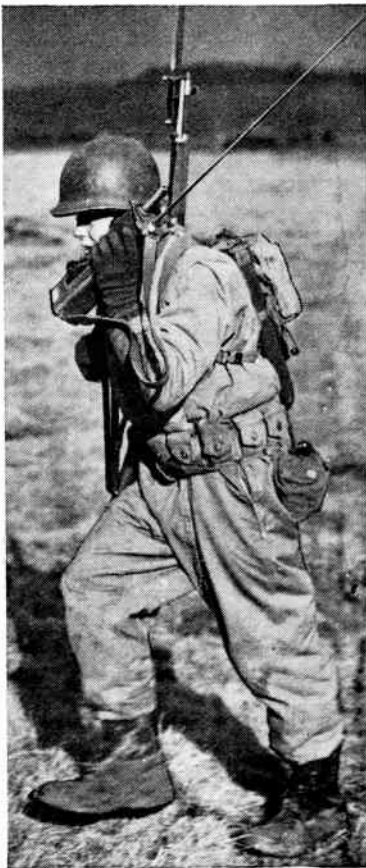
ADVANCING INFANTRY keep in touch with H.Q. by means of the 7-valve "handie-talkie" which weighs about 5lb.
