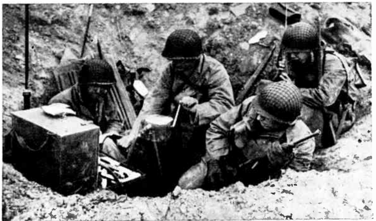
SHELL-HOLE RADIO. A U.S. shore fire control party directing by wireless the fire of Naval guns during the Normandy landings. Note the hand-driven generator. The operator on the right is using a "handie-talkie."
