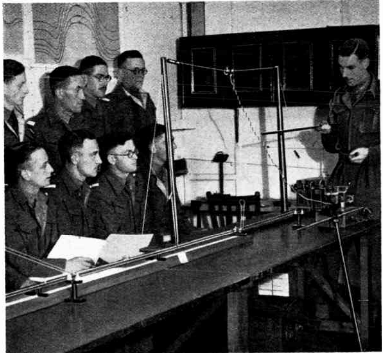
Aerial Demonstration Room. Cadets being instructed in the use of a twisted-pair feeder to a half-wave aerial.
