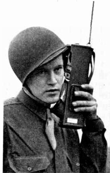
The send-receive switch on the "handie-talkie" is on the side of the 14in. case.
