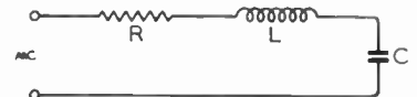
Fig. 1. Conduction current where free electrons are available: displacement current in C even if no conductivity. Both kinds contribute to the magnetic "curl" in the Maxwell equation.
