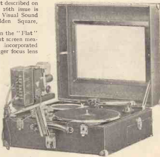
The "Audi-Vision" automatic lecturer projects "still" pictures from 35 mm. film with sound commentary or accompaniment from slow-running gramophone records.
