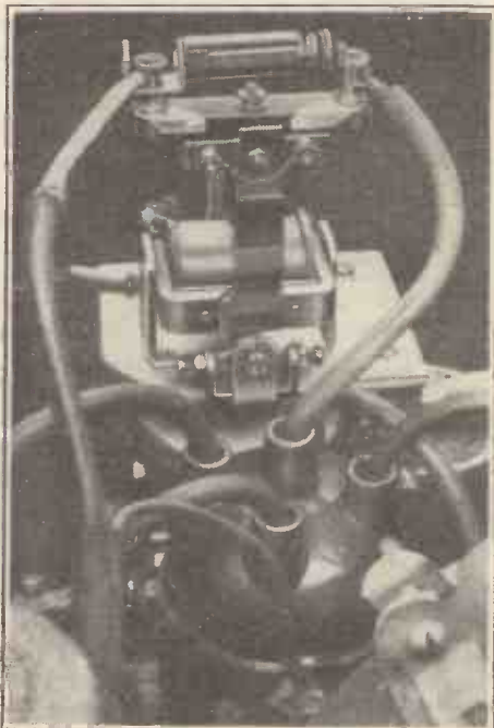
How the relay was mounted on the engine.
