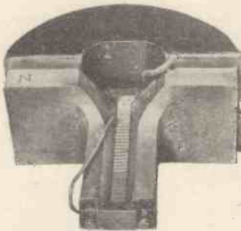
Magnet assembly of a ribbon microphone, as used by the B.B.C., embodying an aluminium-nickel-chrome alloy magnet (Darwins, Ltd.).
