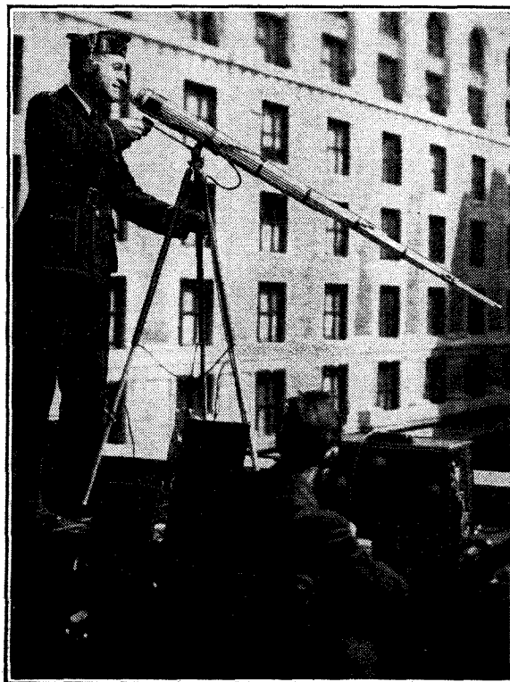
THE "MACHINE GUN" MICROPHONE. Designed for use in outside broadcasts where the level of extraneous noise may be high, this Western Electric microphone is fitted with a bundle of 55 aluminium tubes with lengths which increase in uniform steps from 1½ ins. to 5ft. Each tube is sensitive to one particular frequency, but the resonances are so close that they merge and the frequency response on the axis is not appreciably modified. Sounds with frequencies above 350 cycles are considerably attenuated outside angles of 60 degrees on either side of the axis and the microphone has also been successfully employed indoors to overcome the effects of excessive reverberation.
