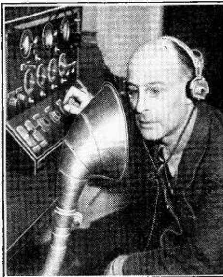
MUSEUM PIECE? The dramatic producer at Milan uses an ordinary speaking tube in preference to its modern electrical counterpart for the purpose of communicating instructions from the control room to his actors in the studios during rehearsals.
