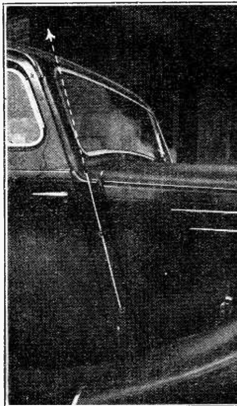
CAR RADIO AERIAL. Fitted just forward of the front door this Philco aerial is only 20 inches long when closed up but can be extended to over five feet when required.
