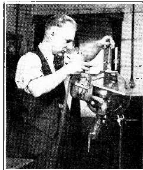
PROGRESS IN TELEVISION is not confined to this country. A television transmitting tube is shown being made in the Philco factory in America.
