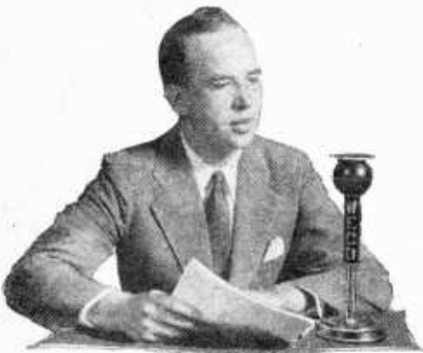
The latest Western Electric studio microphone which has been specially designed not only to have equal sensitivity but also a uniform frequency response for sounds arriving from any direction.
