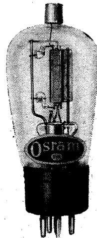
Fig. 3.—A valve voltmeter triode, with high input impedance at radio frequencies.
