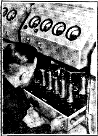
The rapidly approaching debut of the Alexandra Palace transmission adds interest to this illustration of the modulation unit of the Berlin television transmitter.
